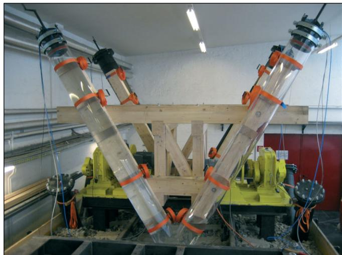
Fig. 1: Liquid-V-Damper made of Plexiglas mounted on the testing bridge designed by the Institute for Structural Engineering – Steel Constructions, Vienna University of Technology
