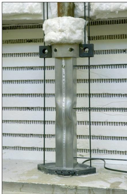
Fig. 2: Welded square hollow section after the compression test at elevated temperature
