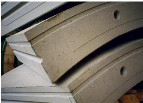
Figure 3: Chamfer design for one- pass segmental lining on the project RER Line EOLE, Lot 35B in Paris, France in 1993 [1]
