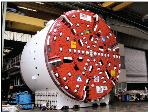
TBM WITH D_{EXC} = 10.60 M IN MANUFACTORY HALL
