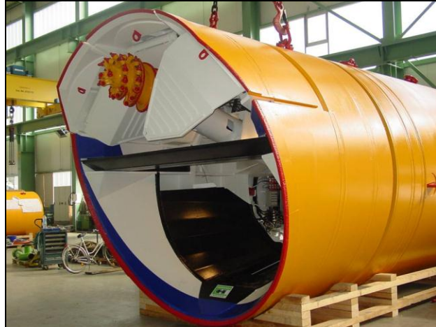
TBM OPEN SHIELD MACHINE, D_{exc} = 3.74 M
