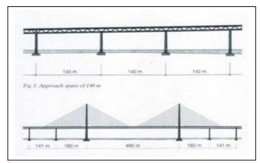
LONGITUDINAL SECTION OF THE HIGH AND APPROACHING BRIDGES.
