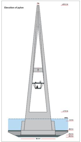
Fig.4 : The cross section of the pylon of the cable-stayed bridge [www2008].
