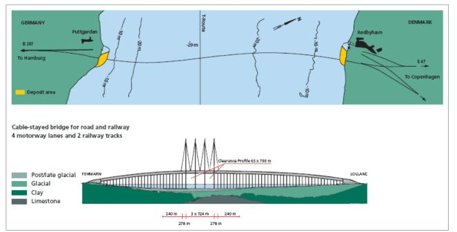
Fig.3: Layout and longitudinal section of the cable-stayed bridge option for 4 motorway lanes and 2 railway tracks [www2008].
