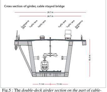
1g.5 : The double-deck girder section on the part of cablestayed bridge [www2008].
