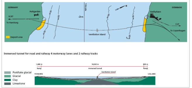
Fig.6: The: Layout and longitudinal section of the immersed tube option for 4 motorway lanes and 2 railway tracks [www2008].
